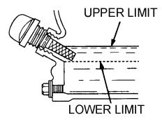
Figure 7. Engine Oil Dipstick(Oil Level)
